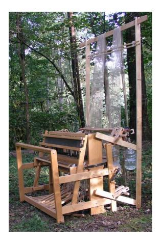
The trapeze can be used with a table loom by clamping BOTH the trapeze and the loom to the table.
