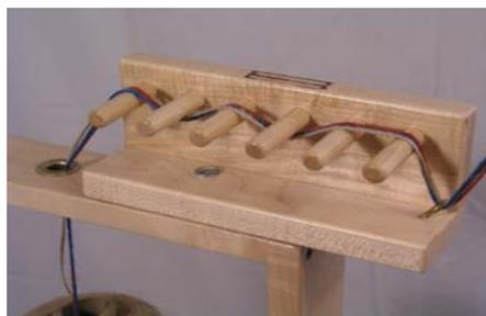
Wind your warp with ease. Six dowel pins, Which have been hand-sanded to a smooth finish, allow the appropriate tension for your warp or bobbin. The tension box can be used alone or attached to our Doubling Stand.
