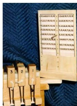
A handy device that clamps to any loom on which can be written the treading order for your work. A Stainless steel pin is moved along in pre- drilled holes to mark your place.
