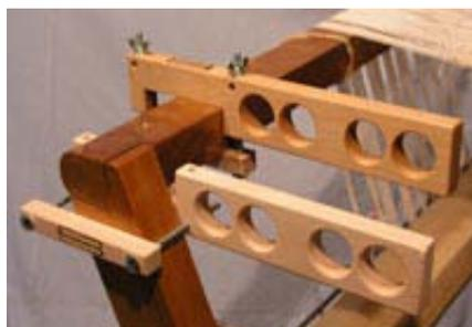
Some things are heaven sent! You absolutely must own a pair of angel wings. The wings clamp to the front or rear beams and hold your lease sticks while warping and/or weaving. The wings are made to accommodate round or flat lease sticks.
